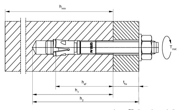
$egin{array}{lll} h_{ef} &=& Effective anchorage depth \\ t_{fix} &=& Thickness of fixture \end{array}$
